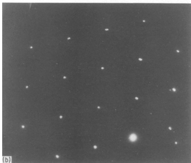
Figure 4 (a) High-magnification image of typical hexagonal platelets of \alpha -beryllium, and (b) a diffraction pattern of a hexagonal platelet is also shown.
